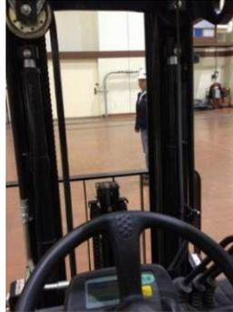
**Fig. 12.** Real world scenario where forklift operator has obstructed view caused by forward forklift bars. (D2000 Safety, 2014)
